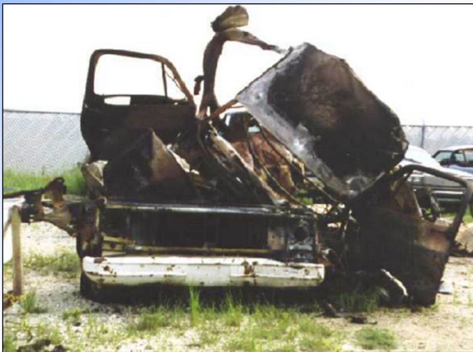
Truck after LOX tank explosion
